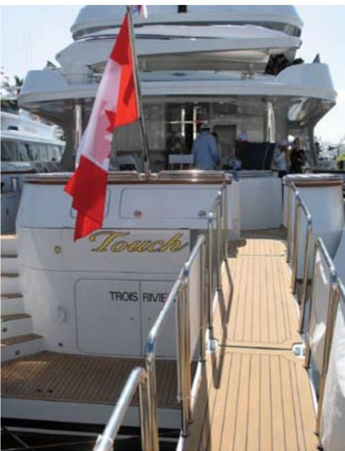
**Flexiteek is supplied** ready to lay. All our decks are custom made from templates for each project. We supply them in one piece ready to glue down, complete with margins, hatches and deck details.
